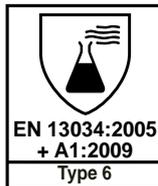
clothing for limited use (type 6). Chemical protective suits (type 6) cover and protect at least the torso, such as one-piece overalls and two-piece suits with or without a hood and with or without socks or overshoes.
